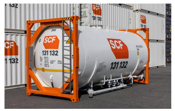
Top: Tank and connections fit inside ISO footprint
