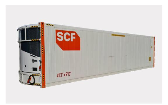
Top: SCF's 41ft Refrigerated Container is built with super thermal properties to reduce machinery run time.
